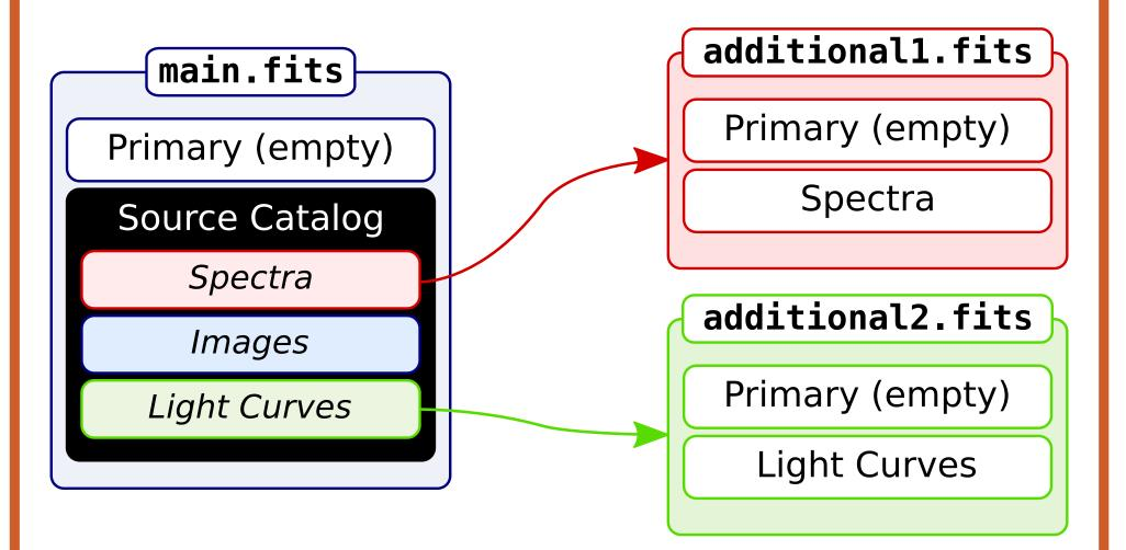
References to additional data must be provided in the form of the *FITS* extended filename syntax (see example). The Primary extension in the main *FITS* file and every additional file may either contain source image data or should be empty.
