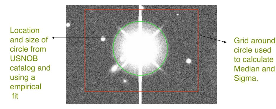
Replace the pixel values in the circle with Gaussian noise with mean and sigma that of a square grid around the circle
