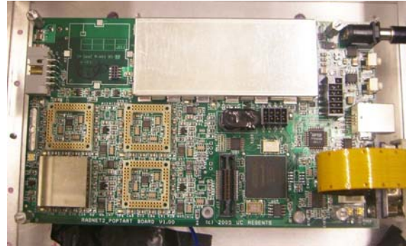
Fig. 4 DCU test setup using a “poptart” board. This can accommodate 4 DCUs and control them through an Altera Cyclone FPGA. The board contains HV PS circuit shielded in an Al case.
